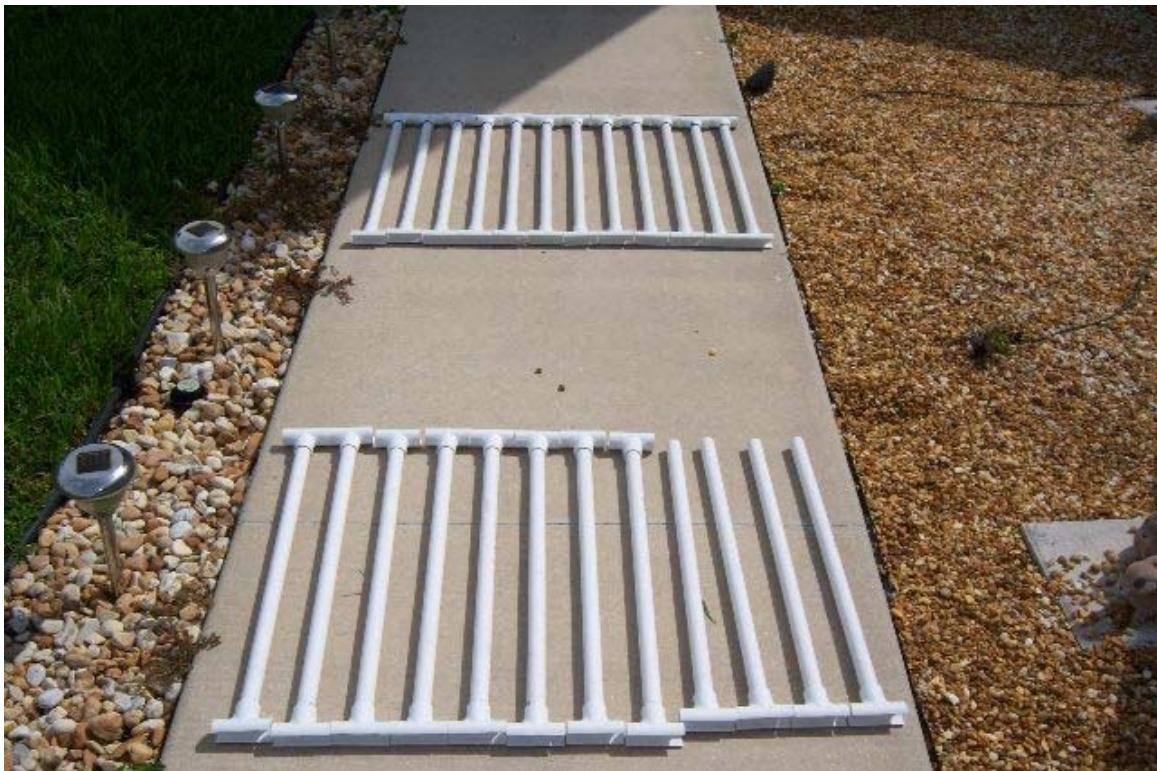
**16. Now it is time to make your 24" VERTICAL SUPPORTS. Same as above, Glue a snap on tee onto ONE END ONLY, lay them on a flat surface, attach the other tee, mark it and THEN glue the other snap on tee in place.**
