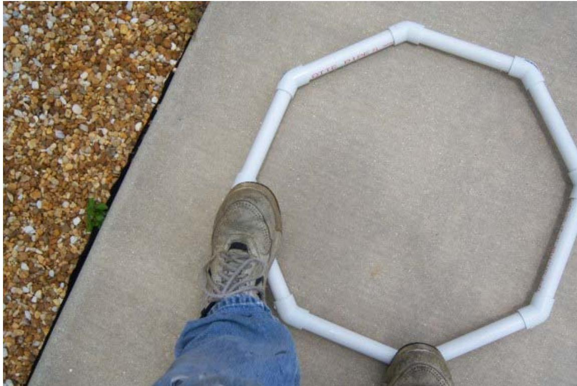
**4. These have to be as STRAIGHT AS POSSIBLE. Using your foot, simply apply pressure until all the elbows are touching the ground and your octagons are straight**
