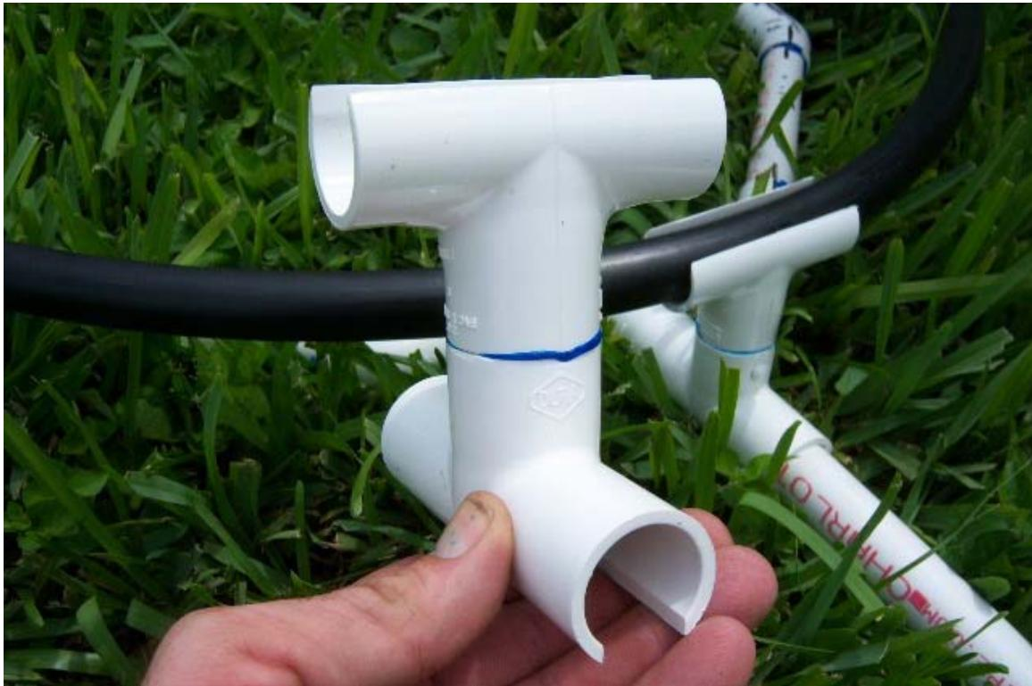
11. Now it is time to make the TRUNK RING. Take one (1) Dura Tee and (1) Spears Tee and insert (1) of the 1.5" pieces of 3/4" PVC Pipe gluing it into one end. Now MAKING SURE THE OTHER TEE IS PERPENDICULAR to the first one, glue it on the other end of the 1.5" piece of PVC Pipe. Do this (12) times. (Set 4 aside for step 15)
